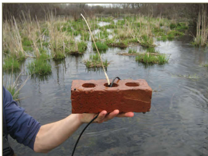
Photo 69. Passive data logger receiver used to record turtle passage at culvert on highway 24. ©K. Gunson
